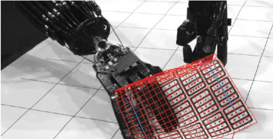
Top view of the calibrated five camera setup / anthropomorphic robots hands interacting with paper.
