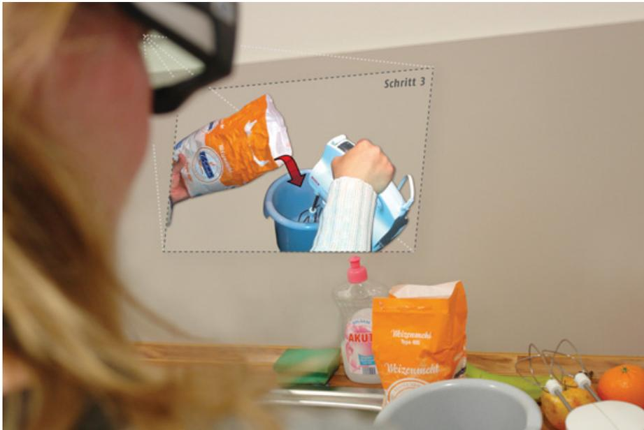
*Adamaas offers individualized assistance, for example when mixing cake batter. The virtual field appears directly in front of the user's face.*
